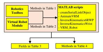
Figure 4. Schematics of implementation of VRM\_Robot class in MATLAB
