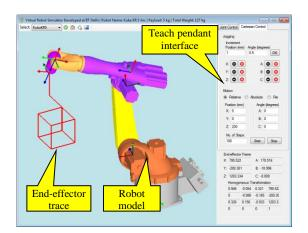
Figure 2. User Interface of Virtual Robots Module in RoboAnalyzer
