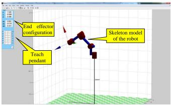
Figure 1. Skeleton Model of KUKA KR5 Arc in Robotics Toolbox
