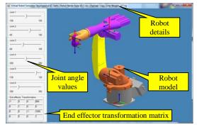
Figure 5. VRM Visualization add-in launched from MATLAB
