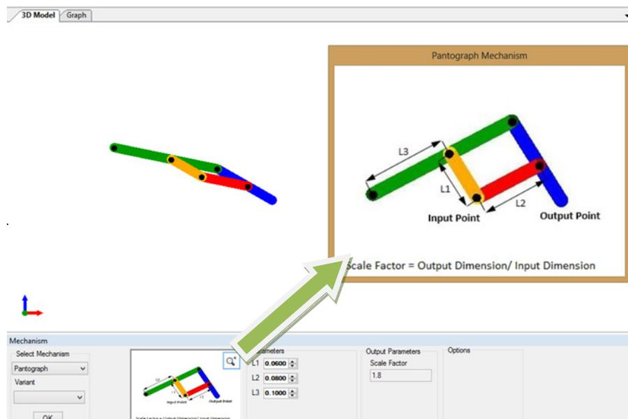
Figure 2: Mechanism description window opened by clicking the zoom button.
