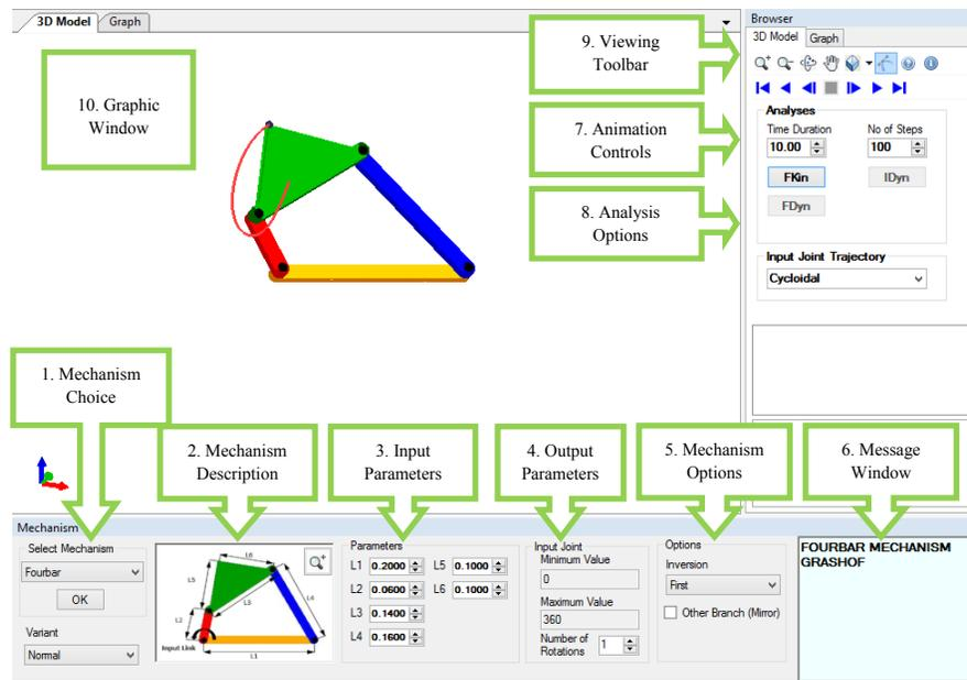
Figure 1: The user interface of Mechalyzer v3.
